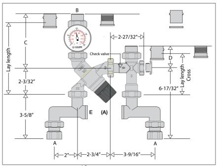
(A) This kit provides one pivot connector with a  $^3$ 4" FNPT port (E), which can be used for applications where there is no pressure relief valve on the tank. Install that pivot connector on the hot side to add a pressure relief valve. For applications where a pressure relief valve is present on the tank, install the pivot connector with the FNPT port on the cold side for incorporating an expansion tank.
