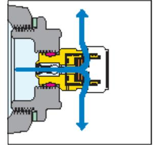
The **manual** discharge position is achieved by unscrewing the knob approx. one turn. Typical use of this method is when refilling the system.
