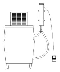
Plug the provided AC/DC adapter into a working electrical outlet to turn on unit. The blue light on the front will turn on indicating normal operation. NOTE: The ActivePure® cell needs to be replaced if the blue light remains off.
