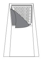
3. Install Velcro strips to the inside vent just outside of the holes. Attach Optional Prefilter by pressing smooth side of pad firmly to Velcro.
