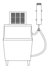
Cut remaining of hose to size, attach to splitter and insert into the two bulkhead fittings in the ice machine.
