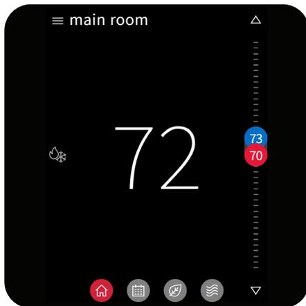
A simple, central **home screen** displays the current temperature, the current mode, and a slider for adjusting the temperature. Users can also adjust the set point using the arrows. The top-level screens are accessible through icons at the bottom of this screen.
