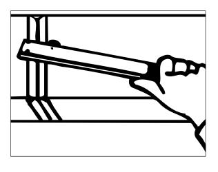
Grasp adjoining duct flanges with wheels of Duct Stretcher to **pull sections together while installing drive cleat** with free hand.
