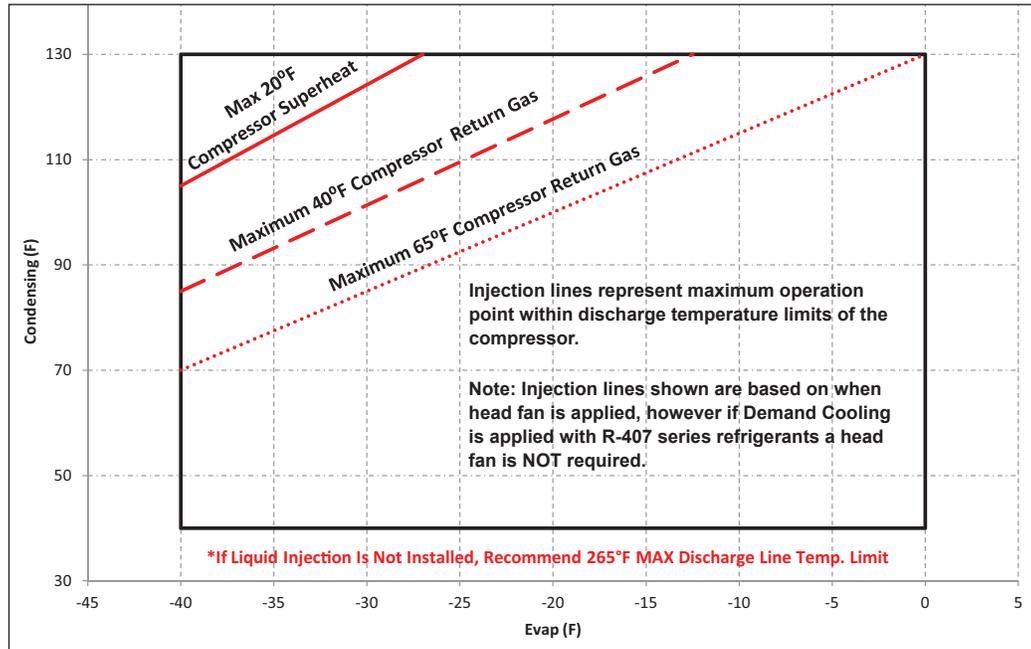
**Figure 2 – Low Temperature Operating Envelope with Demand Cooling for R-407A, R-407C and R-407F**
