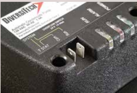
Overflow Safety Switch
