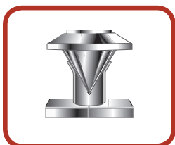
Flares rolled out above die bar.
