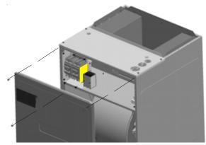
Install the four SPW-01 kit wires to the circuit breaker lugs and torque lug screws to 35 in-lbs. Ensure all wires are tucked inside the control box.
