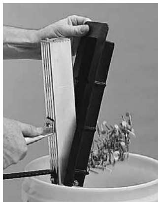
Quick Release Sleeve allows debris to be easily removed.
