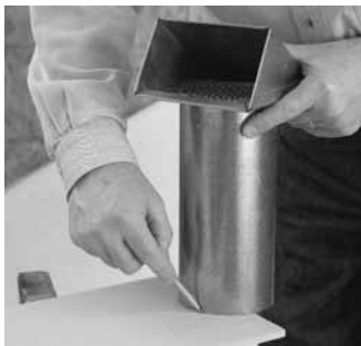
Mark the arc of outlet diameter to be removed from plank.
