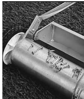
Quick Release rotates housing toward hopper.
