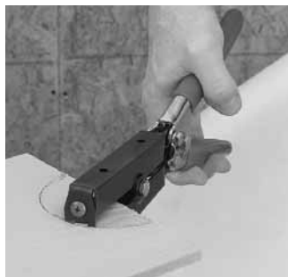
Use Notcher to score along marking to avoid fractures outside arc.
