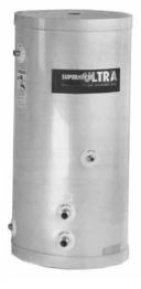
The Super Stor Ultra is true advancement in hot water generation. By tying the Ultra into your existing or new boiler as a separate zone with a circulator or zone valve, it will start the boiler only when the Ultra requires hot water and transfers heated energy through the high output heat exchanger to produce larger amounts of hot water.
