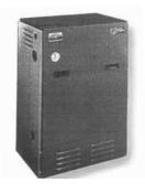
The UB90-100 offers a remarkable 90% AFUE efficiency rating, dramatically reducing fuel consumption and paying for itself in substantial fuel savings. The UB90-100 features integrated boiler control with high limit for operation, safety and diagnostics. Ignition is provided by a hot surface igniter and single stage gas valve. The UB90-100 has sealed combustion, direct-vent forced draft design to draw fresh air from outdoors for combustion, instead of from inside the home.
