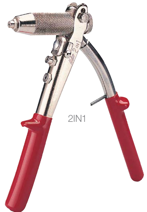
SHORT "RATCHET ACTION" POWER STROKE Bolt in lower hole for hard pulling rivets in several easy pulls.
