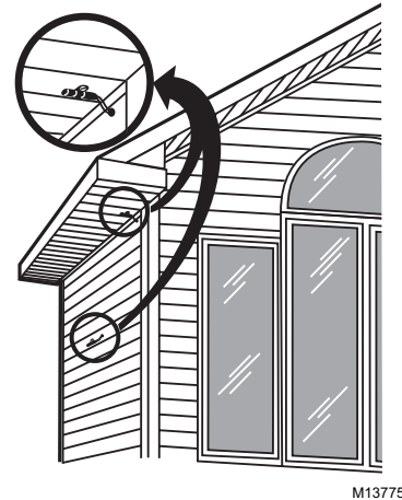
Fig. 7. Outdoor temperature sensor installation.
