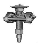
Sporlan Type M valve is a cast bronze body, externally adjustable valve with either ODF solder or FPT flange connections. The thermostatic element is replaceable, and the inlet connection has a permanent 12 mesh strainer. This valve type provides capacities greater than the Type H, and it is designed for both air conditioning and refrigeration applications. Flanges for the Type M valve are interchangeable with the Type V.
