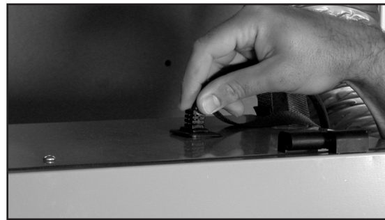
Figure 17 Insert the power cord on top of the unit. Press firmly to make sure the power cord is secure.
