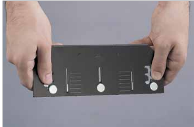
3/8 in. (9.5 mm) and 1" (25.4 mm) folding depths
