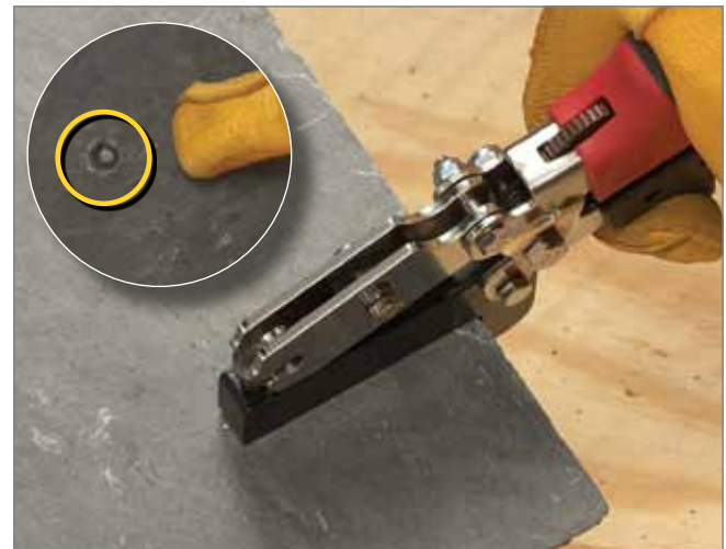
Clean Recessed Nail Holes
