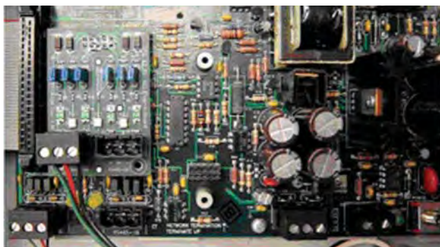
Figure 2.6 CoreSense Diagnostics Network Interface Board
