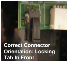
Orientation of communication harness connector
