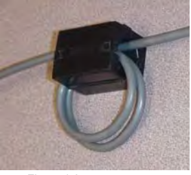
Figure 1.0 Fair-Rite Filter Installed on RS-485 Communication Line
