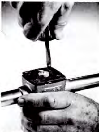
2—Remove the 4 Screws from hold down plate
