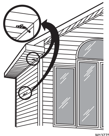
Fig. 7. Outdoor temperature sensor installation.
