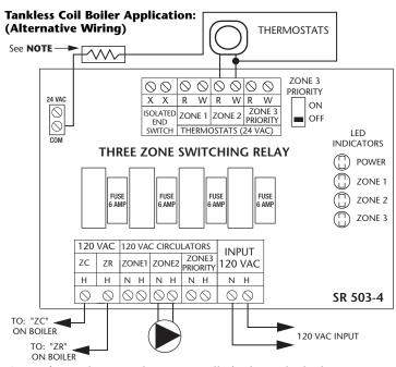
**Operation:** When any thermostat calls for heat, the boiler is given a signal to start. The appropriate circulator is energized only when the boiler temperature is above the set low limit.
