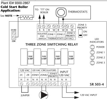
Operation: When any thermostat calls for heat, the appropriate circulator is energized and the isolated end switch (X and X) will start the
