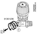
To remove the theft protection use screwdriver 013G1236 and screw into the hole (1). Pull out until the stop is reached (2).
