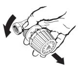
To remove the thermostat turn the base counter-clockwise. This will also reset the the snap-action mechanism when an audible "click" is heard.
