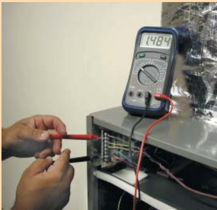
The New SUPCO DM25 digital multimeter being used to troubleshoot an electric furnace.
