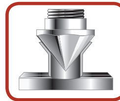
Flares rolled out above die bar by super-smooth faceted cone. Makes stronger, highly polished flares.
