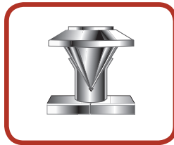
Flares rolled out above die bar.
