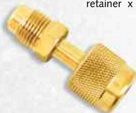
PART # CD2090 PKG QTY: 1 90° 1/4" female flare retainer x 1/4" male flare.
