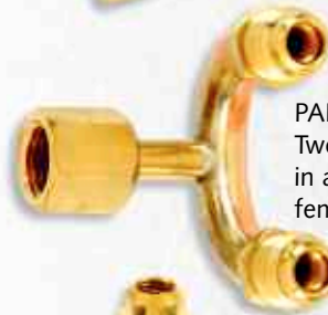
PART # CD8725 PKG QTY: 2 The CD8725 has a gasket in the 1/4" hex nut. The valve body is stationary. When threads of existing system fittings are stripped and a new core won't go in, use this. It has a core and no depressor tip.
