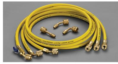
The new A2L refrigerants, R-32 and R-454A, have adopted left-handed connections for their tanks. These new refrigerants are categorized as slightly flammable, so left-handed connections were implemented to differentiate them from A1, non-flammable refrigerants. As the industry adopts these new refrigerants, **YELLOW JACKET® A2L Tank Adapters and Charging Hoses** incorporate left-handed connections so a service technician can safely charge A2L refrigerant systems.
