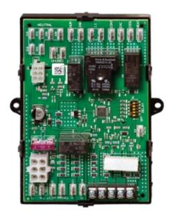
On the surface, the job of the ST9120U1011 is very simple: monitor temperature demands and run the fan as needed, but the ST9120U1011 also handles all the little complexities of the job. And best of all, it's ready to work in just about every situation, replacing more than 41 other models.
