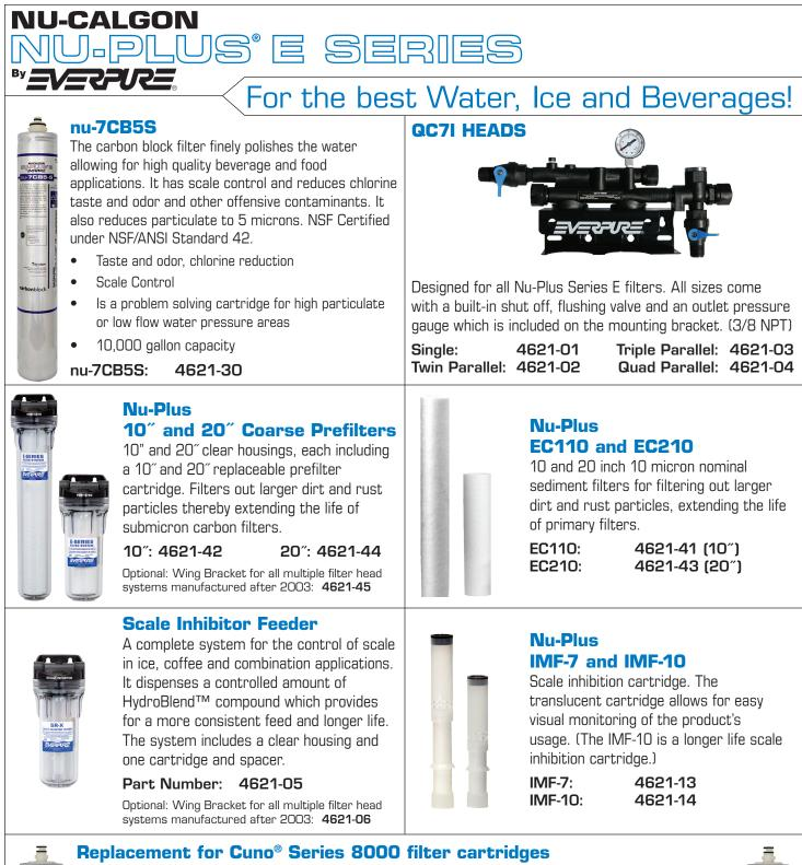
The Nu-Plus E Series CU-S and CU cartridges are equal replacements for the CUNO Series 8000 filter cartridges in food service, vending machine and OCS applications. Both incorporate a carbon block filter that polishes water for high quality beverage and ice, reducing chlorine tastes and odor and other offensive contaminants. They also reduce extra fine dirt as small as 5 microns. Additionally, the CU-S provides for the reduction of scale formation.
