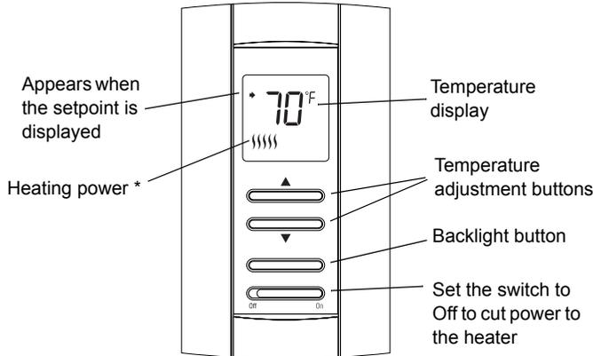
\* The thermostat displays the heater duty cycle required to maintain the desired temperature. For example, if the heater is activated 40 percent of the time, is displayed.
