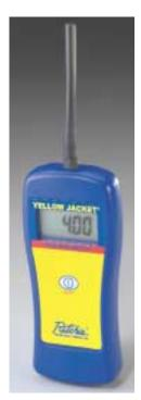
The unit benefits all contractors who wish to eliminate the mess and fragility of U-tubes or diaphragm type gas pressure gauges. This easy to use electronic instrument provides a continuous display of the measured positive or negative pressure. The unit provides
