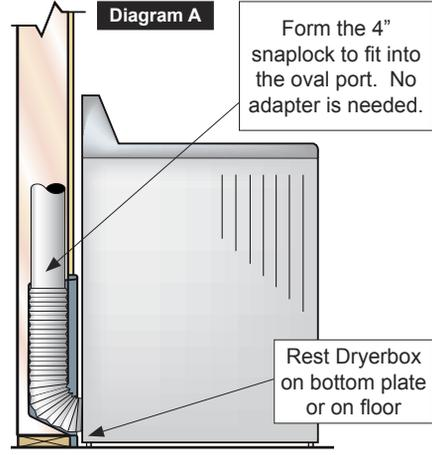
Install box as low as possible and as near to the center of the proposed dryer
