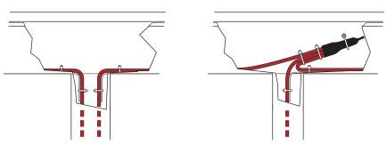
Figure 10 Heating cable at top of downspout
