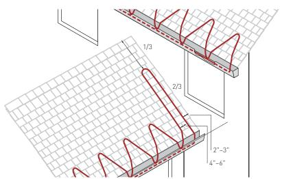
Figure 8 Layout for a roof/wall intersection
