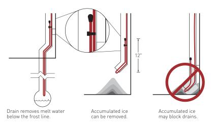
Figure 11 Heating cable at bottom of downspout
