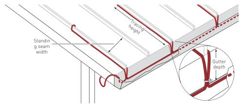
Figure 4 Layout on a standing seam roof
