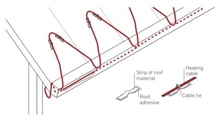
Figure 14 Belt loop approach on a sloped roof
