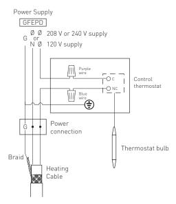
Figure 17 Typical controller wiring—single circuit
