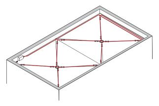
Figure 15 Belt loop approach on a flat roof
