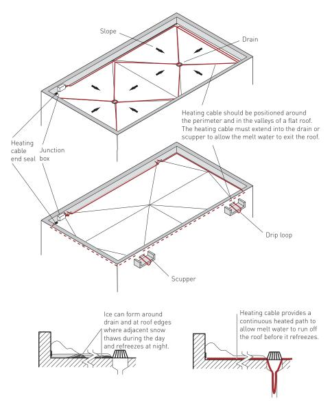
Figure 5 Layout on a flat roof
