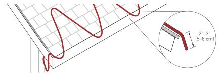
Figure 6 Layout for heated drip loops
