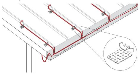
Figure 13 H913/H914 clip on standing seam roof
