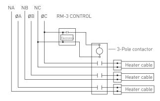
Figure 18 Typical wiring diagram using a RM-3 controller-multiple circuits
