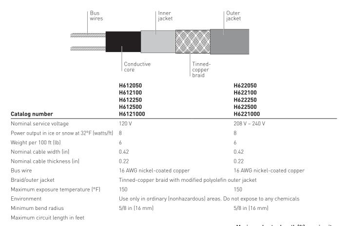
Maximum heater length (ft) per circuit for minimum start-up temperature Circuit breaker Heating cable type 0°F 32°F rating (Amps) WinterGard Wet H612 15 100 125 120 Vac 20 125 165 30 150 200 WinterGard Wet H622 15 200 250 208 V - 240 V 20 250 30 305 400
