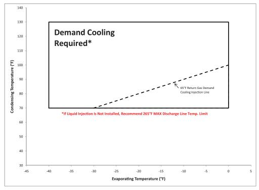
Figure 3 – Low Temperature Operating Envelope for R-22 at 65°F Return Gas (with Head Fan)
