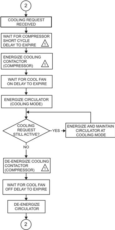
⚠ THE OPERATION IN THE BLOCK IS SKIPPED WHEN A SYSTEM WITH A CONVENTIONAL THERMOSTAT IS USED. THE OPERATION IS PERFORMED IN SYSTEMS WITH AN ENVIRACOM™ THERMOSTAT ONLY.
