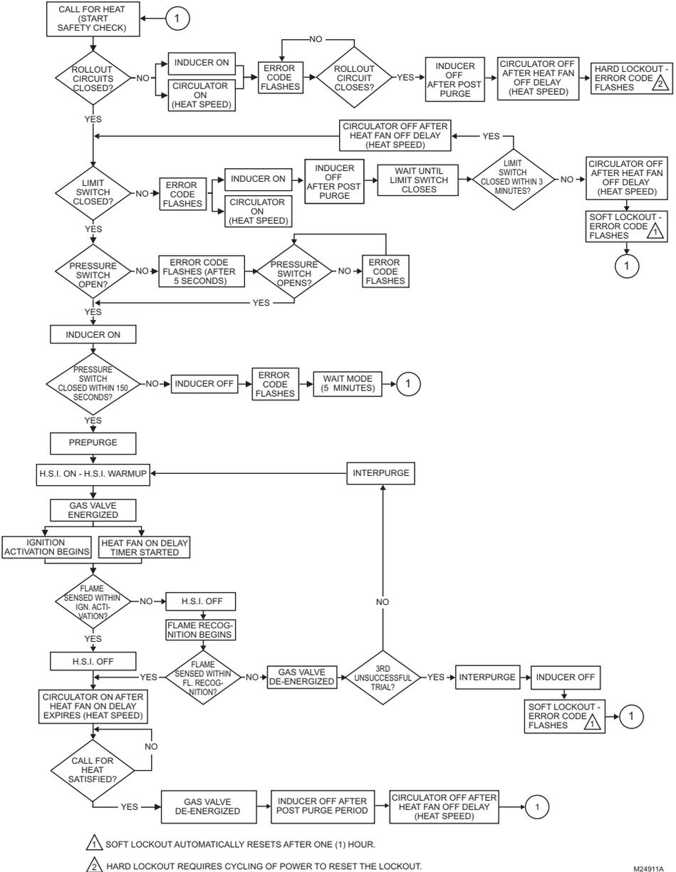
Fig. 9. S9200U1000 sequence - Call for Heat cycle.
