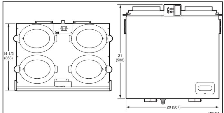
Fig. 1. Dimensions in in. (mm) and clearances.
